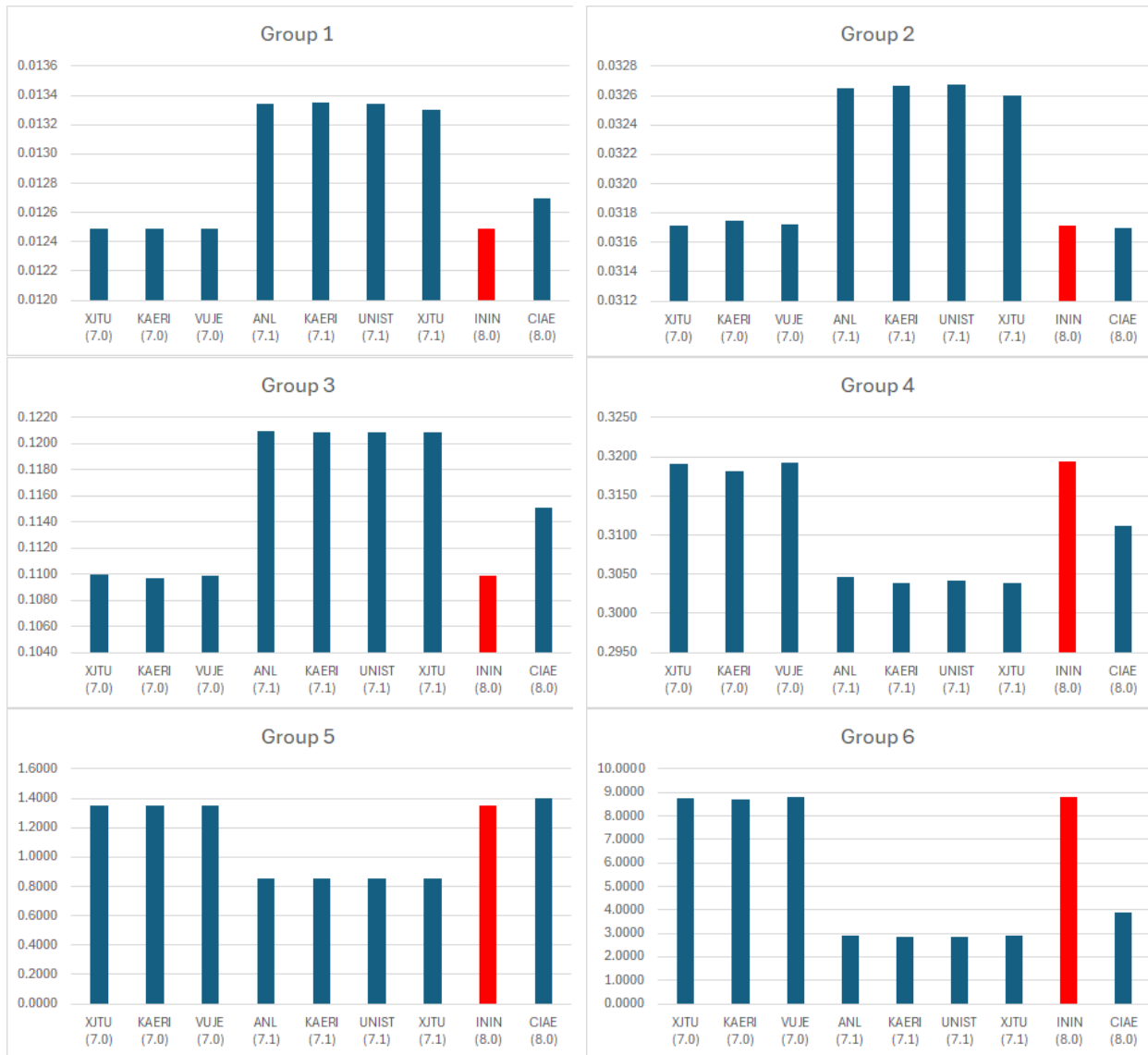
Figure 6. Decay constants \lambda_i [sec -1 ] for different delayed neutron precursor groups
