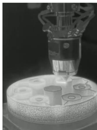
Figure 2. Use by ORNL of thermal imaging to monitor direct deposition of stainless steel to 3D print a reactor component (credit: ORNL)
