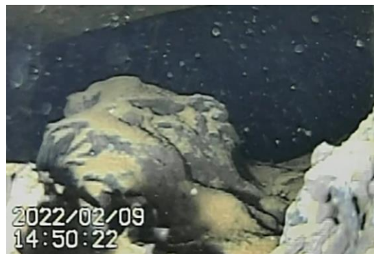
Figure 4. A robot-captured image of melted fuel inside the core of a Fukushima reactor (credit: IRID/Hitachi-GE Nuclear Energy, Ltd.)
