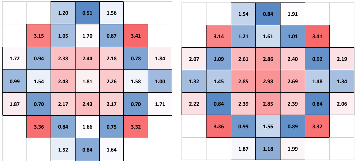
Figure 7. The assembly-based model compares Relative errors with the SERPENT code of radial power distribution for AZTRAN (left) and PARCS (right).
