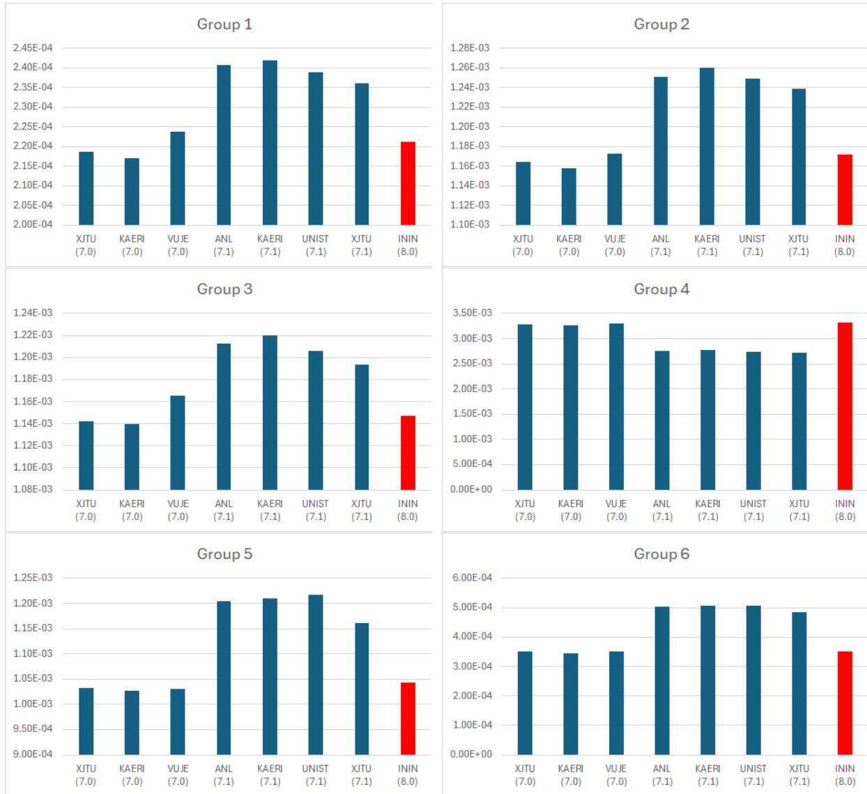
Figure 7. Fraction of delayed neutron precursor groups \beta_i
